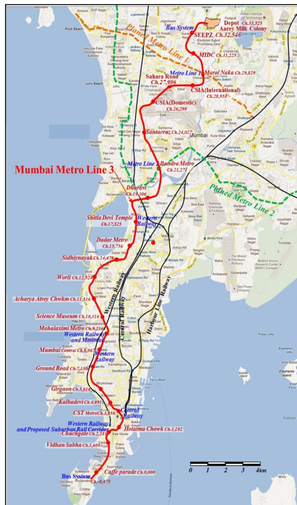
Figure 1: Alignment of Mumbai Metro Rail Line 3
